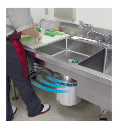
Everything you need to operate more efficiently. Salvajor's patented operator sensor detects the presence or absence of the operator. The Control then adjusts the water flow accordingly, reducing water usage by 80% when the operator is away. In addition, the disposer will power off entirely if the operator does not return to the work area before the adjustable run timer expires.
